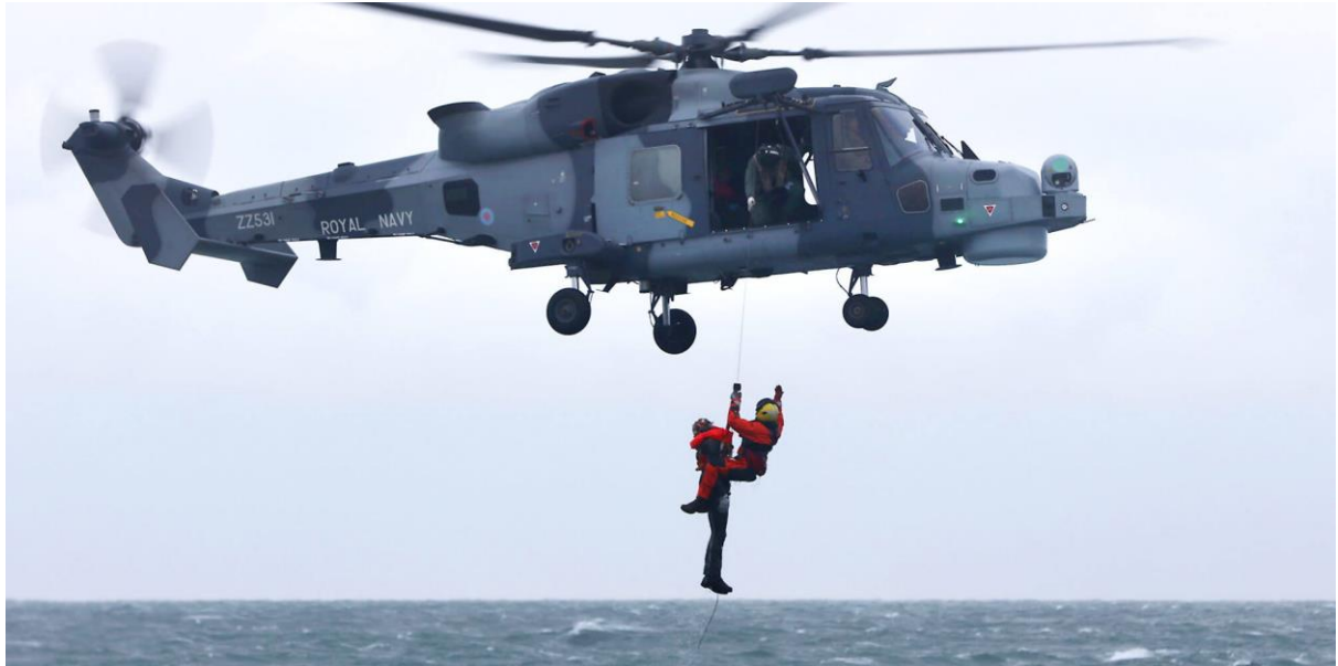
Conducting winching drills off Portland, December 2017. The Wildcat can be fitted with a Goodrich 44316 rescue hoist – with an 88m cable capable of lifting up to 270Kg.
