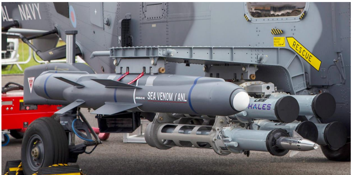
A dummy Sea Venom missile and hermetically sealed Martlet LMMs in their a five-cell launch panner on display at Farnborough. In the anti-surface role, the Wildcat can carry either 4 Sea Venoms or 20 LMM or a mixture of 2 venoms and 10 LMM.
